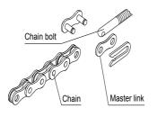
chain box using enclosure master links. Tighten the chain bolt to the bracket with washers and nuts. Pull the chain through the chain wheel box to the other chain bracket at the opposite end of the gate. Connect the other end of the chain and the chain bolt, and then tighten the chain bolt to the chain bracket. Thread up the chain by adjusting the chain bolt. Cut the chain to length if
