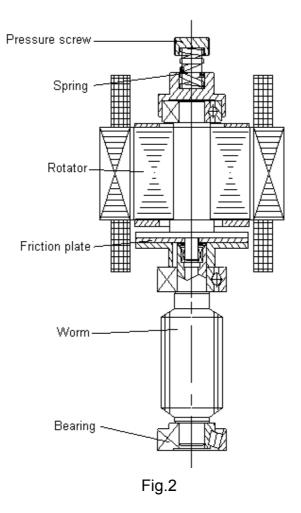
**Release function:** the worm gear components are shown in Fig.3. It includes a pair of plastic gear clutches. In case of power failure you can use the key to release the clutch, and then the gate can be moved manually.
